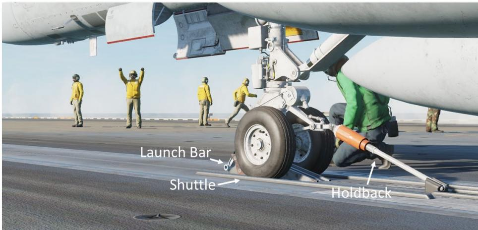
**5. Seat launch bar in shuttle.** When directed, raise the launch bar to seat it in the catapult shuttle. Note that the bar will not fully retract until it is clear of the shuttle after launch.
